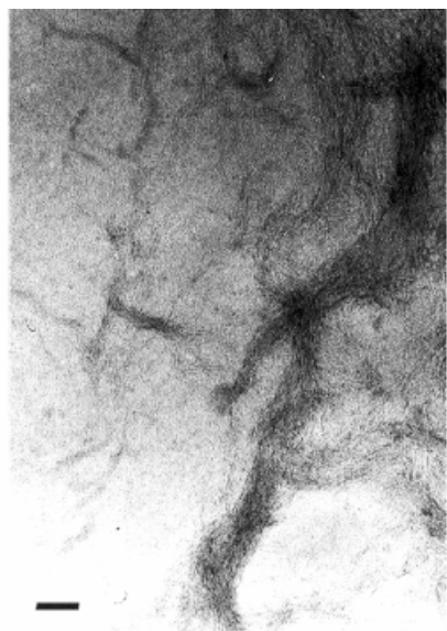
Figure 19. TEM image of poly(LGAGGAG); notice the typical elastin-like fibrous organization; bar represents 100 nm
