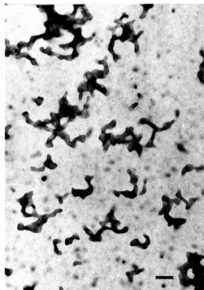
Figure 16. TEM image of poly(LGAGGAG); note the nuclei of diffusion-limited aggregation; bar represents 200 nm
